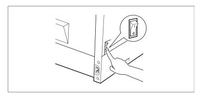
2 Connect one end of the power cord that comes with the printer to the power cord socket. Plug the other end into a power outlet.
