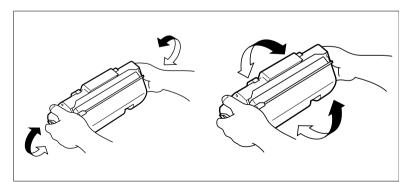
5 Install the imaging cartridge securely into the printer by sliding the pins on each side of the cartridge along the grooves of the cartridge guide.
