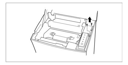
5 Clips secure the exterior side cover from the inside of the printer. Gently maneuver the exterior side cover until the clips release (see illustration).
