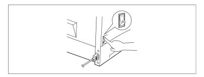
Turning on the printer causes all the indicators on the control panel to light, which indicates that the printer is warming up. In about 23 seconds only the ready indicator remains lit, indicating that the printer is ready to print.
