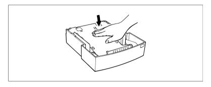
4 Place a stack of up to 500 sheets of paper into Tray 2/Tray 3 so that the side that was facing up when the paper was unwrapped is still facing up.
