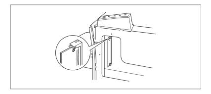
10 Replace the internal side cover using the four screws.
