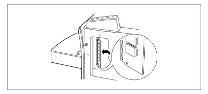
9 Make sure both clips on the socket are pushed through the holes on the SIMM.
