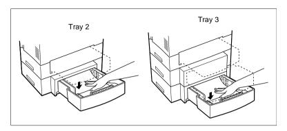
Remove the stack of paper from the tray and pull the misfed paper straight out of the printer.
