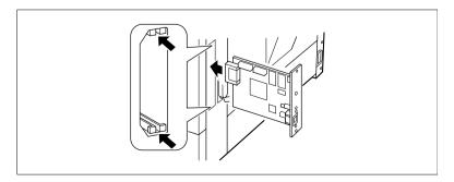
5 Secure the NIC into place using the same screws that were used to hold the cover panel.
