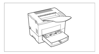
3 Insert the sheet of paper into the manual feed tray with the side to be printed facing up.
