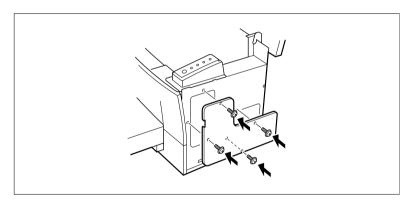
11 Replace the external side cover using the two screws.
